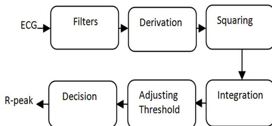
Fig. 3. Pan –Tompkins real time QRS detection algorithm
